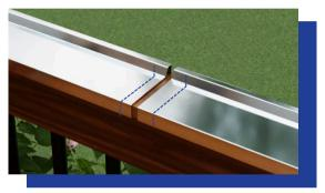
The transition strip features two holes – one along the outer edge and one on the lower inside edge. Secure it using the 1" stainless steel screws with a #2 Phillips screwdriver bit.
