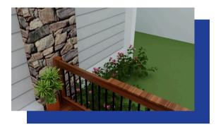
PureSteel Solutions rail onto the 2x6 is not feasible due to space constraints, it is necessary to first uninstall the 2x6.
