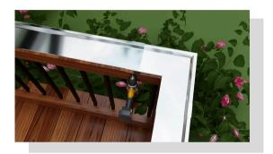
The transition strip features two holes – one along the outer edge and one on the lower inside edge. Secure it using the 1" stainless steel screws with a #2 Phillips screwdriver bit.
